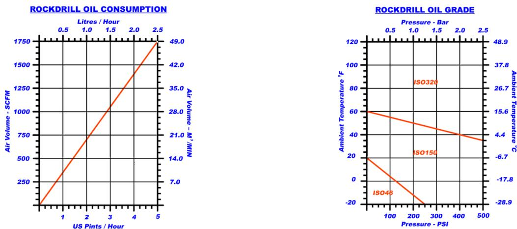
**Remember: Insufficient lubrication or incorrect lubrication grades may result in damage being caused to the hammer and it's components. Hydraulic oils, engine oils, gear oils and diesel are not recommended for lubricating DTH hammers.**
